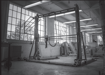
Daedalus Self-built Open Source 3D Printer
